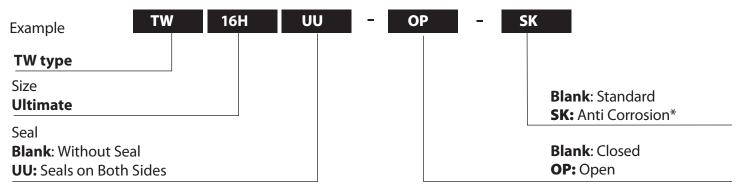
\*For anti-corrosion the load plates are electroless nickel plated with stainless steel balls.
