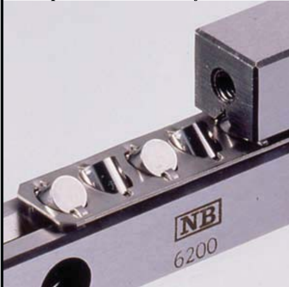
Metal cages hold the rollers via a notch on the top and on the bottom of the rollers.
