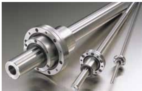
In ball splines, bearings in the nut ride on a grooved shaft that prevents the nut from rotating. This lets it transfer torque. Special versions permit both rotary and linear motion.
