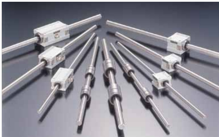
In ball splines, bearings in the nut ride on a grooved shaft that prevents the nut from rotating. This lets it transfer torque. Special versions permit both rotary and linear motion.
